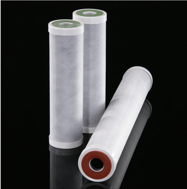
CARBOFLOW MX cartridges are offered in both high efficiency and general grades. They consist of coconut shell sourced carbon, extruded together with an FDA listed thermoplastic binder, to produce an extremely porous yet rigid structure.
