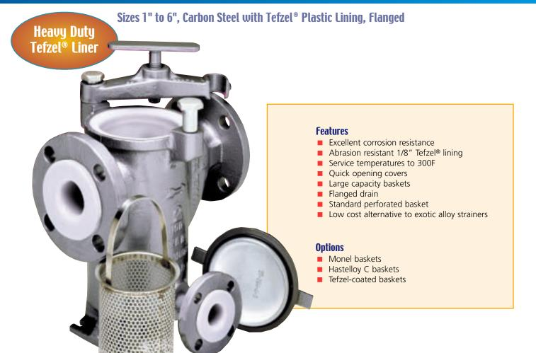
continuous lining of advanced fluoropolymer resin makes the Model 72L simplex strainer an excellent low cost alternative to exotic alloy strainers in a wide variety of corrosive or abrasive lined piping applications. These applications include waste water treatment, paper mills, hazardous materials, flue gas systems, ultra pure water handling, chemical and petrochemical processing. The basic design of the Model 72L is that of our popular, time tested Model 72.
