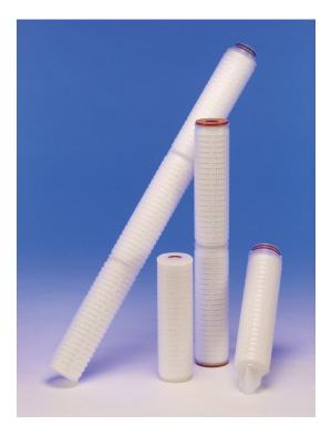
**Tec-Pleat GP Plus** filter cartridges are absolute rated, pleated polypropylene depth filters, they are equally suitable for use as membrane pre-filters or final polishing filters in applications that do not require membrane filtration.
