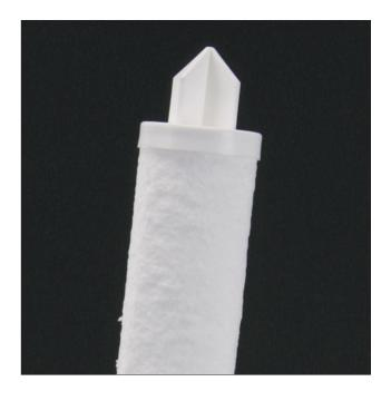
SPUNFLOW QA cartridges are a range of absolute graded density filter elements, manufactured from thermally bonded polypropylene microfibers layered onto a resilient centre core. The construction consists of numerous, distinctive filter zones with coarser outer layers acting as prefilters for the tighter, absolute rated central zone. This profile produces an element possessing high voids volume, for flow rates high flow rates, low pressure loss, high dirt holding capacity and long life.
