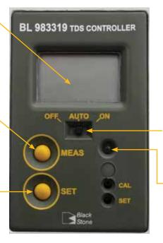
Over-ride Switch. Set to the Auto position for normal operation. Set to OFF to keep Product Solenoid Valve closed, for instance when flushing out cleaning chemicals or for 10 minutes when first installing new membranes. Set to ON to keep Product Solenoid Valve open, for instance when it is desired to override the quality reading from the probe or for troubleshooting.
