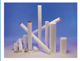
**Tec Spun N** is a nominal rated depth filter cartridge with graded depth filtration, available in Polypropylene to suit a range of applications. Available in a range of Beta Ratio 5000 Absolute micron grades, from 0.5 to 100.
