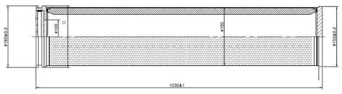
Designed to be dimensionally equivalent to the standard High Flow elements these AWSS TecPleat are designed to fit standard High Flow Housings.
